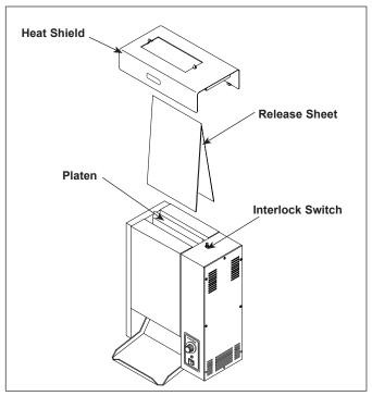
Figure 7. Removing/Installing Release Sheet
